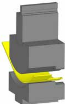
Radius embossing-tool for embossing two lateral straps at the same time
