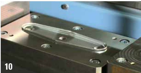
10 Manufacturing a shape in one of the half shells
