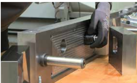
Final assembly of the upper part of the tool
