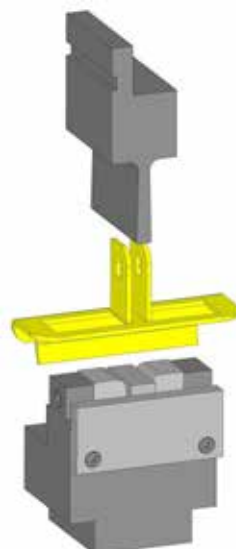
U-bending tool with small inner dimension and cut-out for 90° bend
