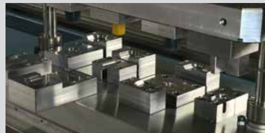
Complete view of pillar-guided special tools for connecting the parts with the individual add-on components
