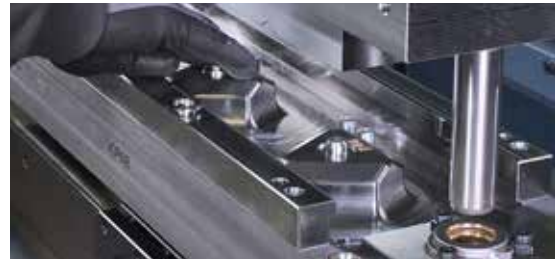
1. step of production: Lay-up of the lower parts of the inner rings in all three stations
