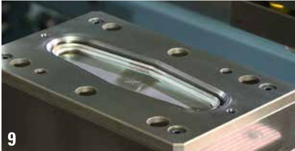
9 Embossing of both half shells (produced in one station)
