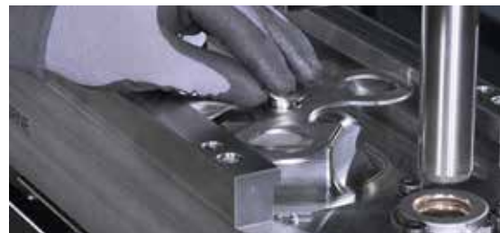
2. and 3. step of production: Lay-up of the plate and the upper part of the inner rings in all three stations
