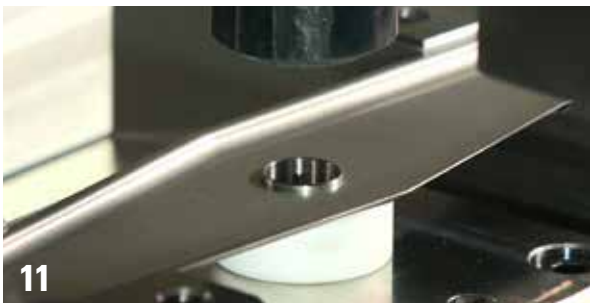
11 Impressing of add-on components with the half shell (inner part)
