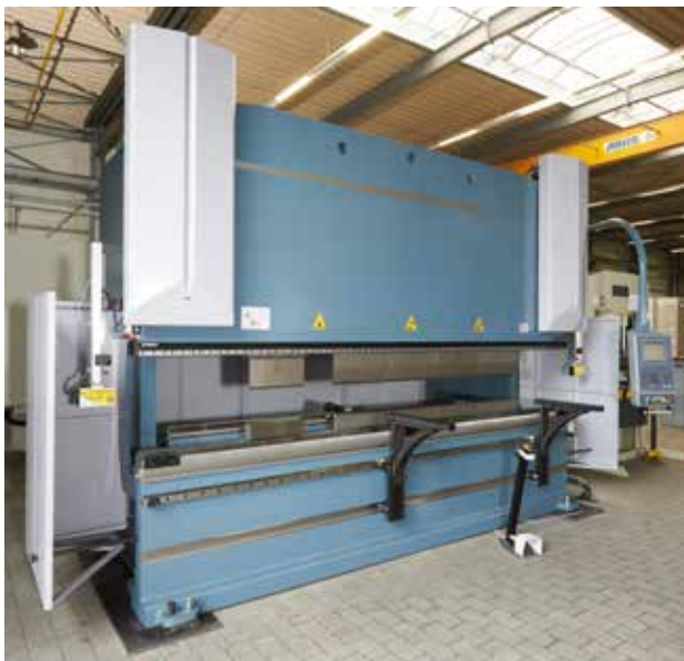
Press brake for test bending L = 4050 mm, press capacity: 3200 kN
