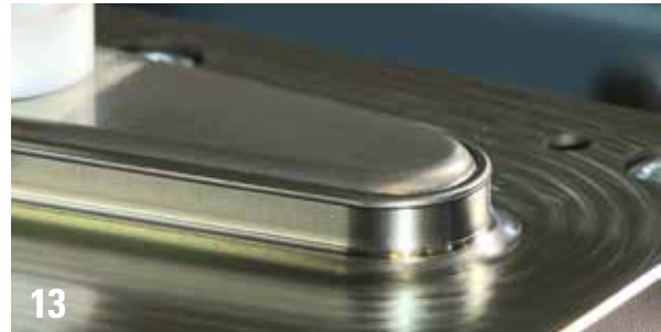
13 Connection of both half shells (inner and outer part) through framed folding
