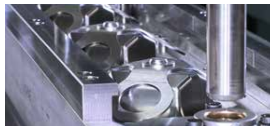
Result in the lower part of the tool - after bending
